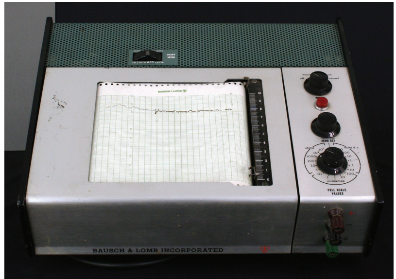
Volt-Ohm-Amp Meter with built in data recorder
