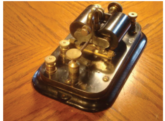
Early armature relay at receive end of telegraph line
