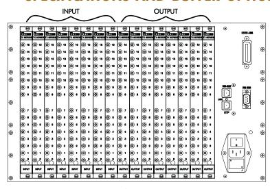
TX/128x128 Mainframe Rear View with IEEE488, RS232 and LAN Control
