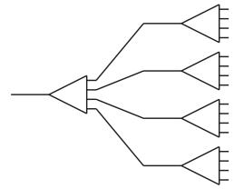
Fig. 2 16x1 Multiplexer using five CXM/4x1 Switches
