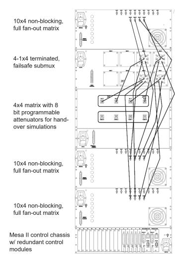
30x4x4 non-blocking, full fan-out matrix with 8 bit programmable attenuators and redundant controls, DC to 18 GHz.
