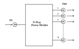
Fig. 7 1: N Power Divider/Coupler
