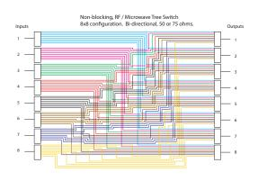
Fig. 1 8x8 Matrix Using Sixteen CXM/8x1 Switches
