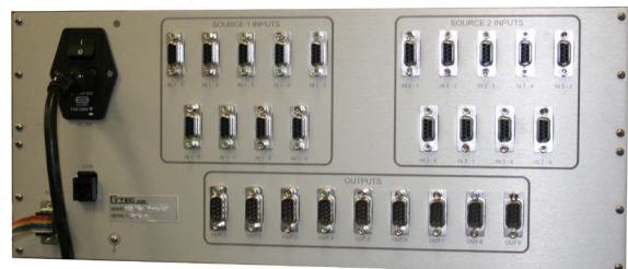
Nine cable A/B group switch using RS9 Switch Modules and D9 connectors
