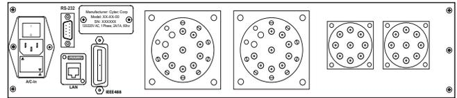
CXM/32 with GPIB, RS232 and LAN Control
