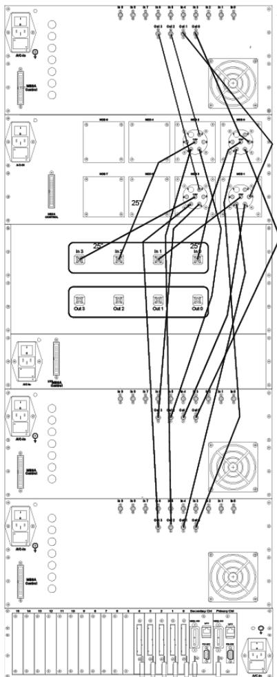
30x4x4 non-blocking, full fan-out matrix with 8 bit programmable attenuators and redundant controls, DC to 18 GHz.
