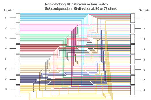
Fig. 1 8x8 Matrix Using Sixteen CXM/8x1 Switches
